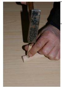
At the beginning, the two 10 mm dowels must be inserted into the holes provided for the 20 mm dowels.
