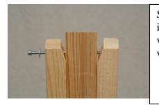
Slide a washer onto the screw, then insert the screw through all three woods. On the other side, slide a washer again and turn a wing nut.
