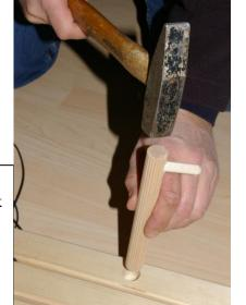
Then also insert the two 20 mm dowels into the holes provided for the pre-assembled disk stand.
