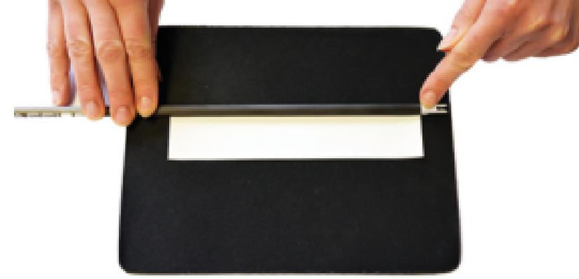
**4. Roll the arrow shaft gently and with a soft pressure over the foil.**
