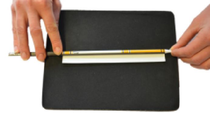
**5. Continue to roll the arrow shaft, till the shaft is completely enclosed by the foil.**
